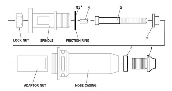
Items in grey are included in the base tool. The item numbers refer to the table in the 'Selecting a Nose Assembly' table below.
